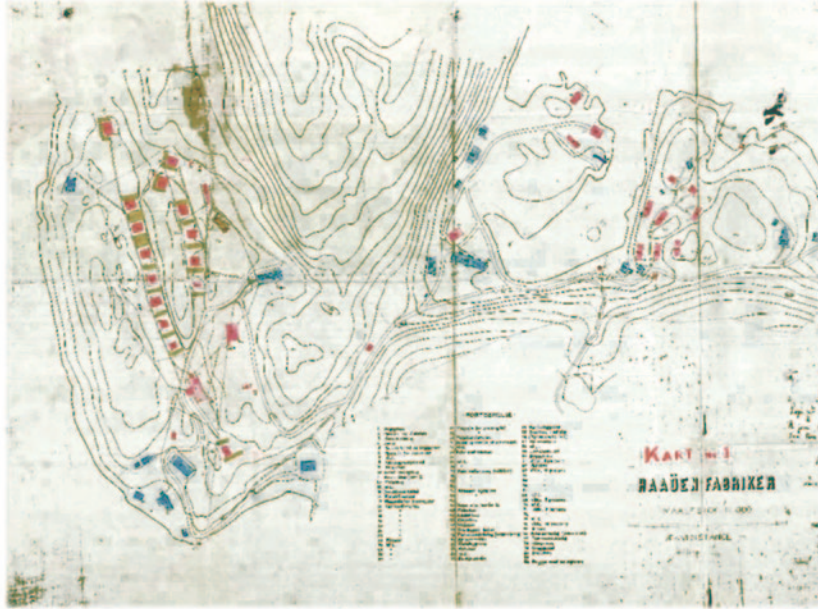
Map of the Håøya dynamite factory in 1916. The two rows of buildings to the west of the area are the buildings described as '8-10 small houses, each located in a small valley, separated by a small wooded hill'. (Buildings marked in red have disappeared). Reproduced with the permission from Frogn municipality.
